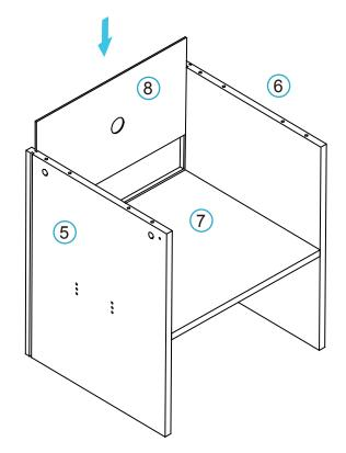
Attach panels [5] and [6] to panel [7] with 4x dowels (C) and secure with 4x locking nuts (B) and tighten with a screwdriver.
