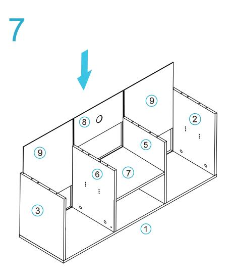
Slide panels [8] and [9] between the grooves of panels [1], [2],[3], [5], [6] and [7] to form the back of the unit, as shown.
