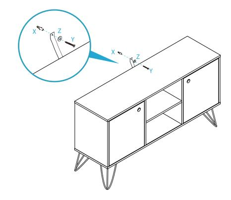
Attach 1x safety strap (V) to the top of the back side of the unit as shown using 1x washer (Z) and 1x screw (W). Tighten with a screwdriver.
