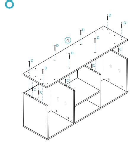
Attach panel [4] to the rest of the unit with 8x dowels (C) and secure with 8x long screws (D) and tighten with a screwdriver.
