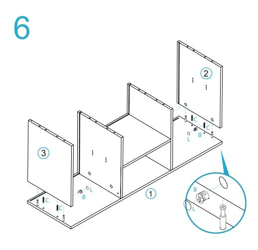
Attach panels [2] and [3] to panel [1] with 4x dowels (C) and secure with 4x locking nuts (B) and tighten with a screwdriver. Seal the holes with 4 x covers (L).
