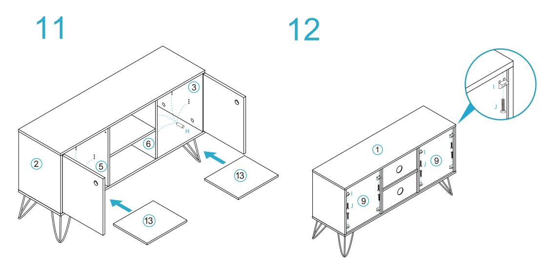
Insert 8x shelf plugs (H) into the end cavities of the cabinet as shown. Insert the shelf panels [13] and balance on top of the plugs.
