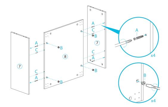
Slot the tray together onto the rest of the table structure as shown. Place 6x locking nuts (B) and 4x dowels (C) into holes. Insert 8x dowels (C) into the top and slot on side panel [4]. Fasten with 12x locking nuts (B) and tighten with a screwdriver.
