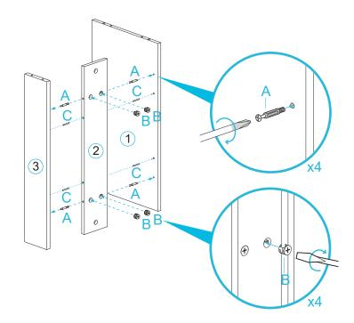
Begin assembly by screwing in 24x bolts (A) into all corresponding holes as shown in both panels [4] using a Phillips screwdriver. Take care not to overtighten bolts.
