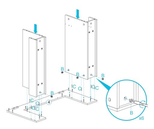
Slot both the components assembled in the previous step together with one panel [4]. Place 6x locking nuts (B) and 8x dowels (C) into holes in the panels as shown an tighten with screwdriver.
