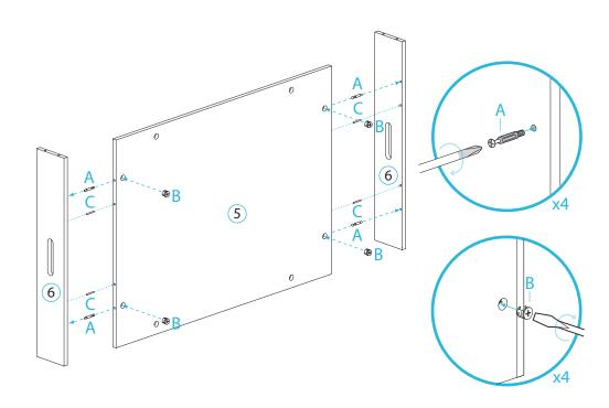
Screw in 2x bolts (A) and insert 2x dowels (C) into holes in each of panels [6]. Slot together with the table panel [5] as shown. Place locking 4x nuts (B) into holes in the panel [5] and tighten with screwdriver.
