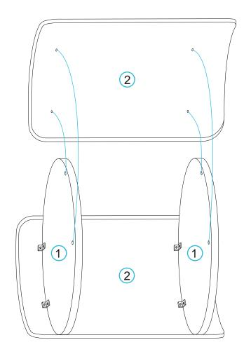
Attach the table tops [1] to a table leg [2] as shown using 4x metal plates (C). Secure using 8x bolts (A), 8x spring washers (B) and tighten with the allen key (D).
