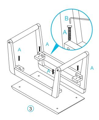
Attach 2 x legs [A] and 2 x arms [2] together and secure with 4 x bolts (A). Tighten with an Allen Key (B).
