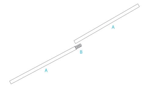
Attach 1x connector (B) to 1x pole (A).
